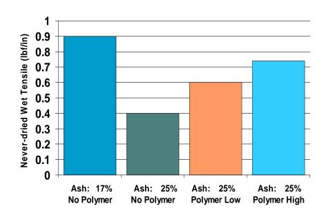
The use of the strength resin can help maintain wet-end productivity at high filler content
