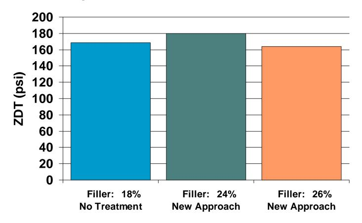
ZDT was used to assess internal and surface strength of paper. This new high ash program enables to maintain this property
