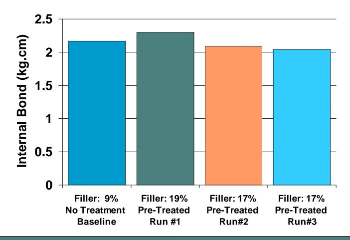
8% filler increase provides significant savings to the mill while maintaining key paper properties
