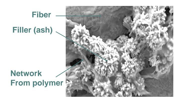
Once the paper is formed with the program components, a polymeric network is created between fibers and fillers
