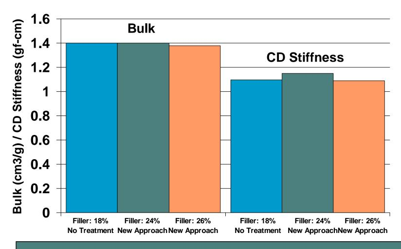
CD Stiffness is critical paper characteristic for copier runability, maintained under high filler loading
