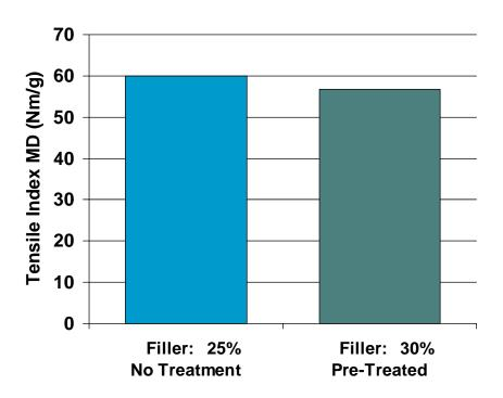
Both bulk and tensile were maintained within specifications
