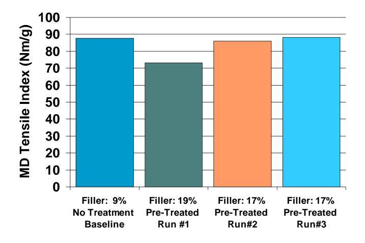
MD Tensile maintained: good paper machine productivity and coater operation were maintained
