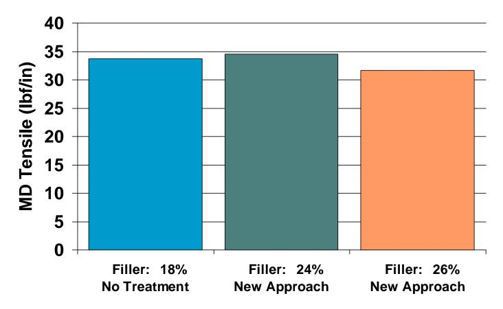
Tensile maintained under high filler loading; MD tensile is important to maintain dry-end paper machine productivity
